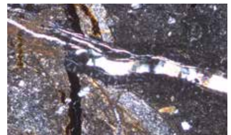
Concrete suffering from cracking induced by ASR.
