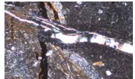
Concrete suffering from cracking induced by ASR.
