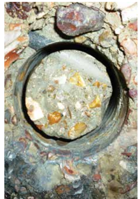
Core sample extracted for laboratory testing.
