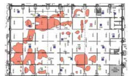
Visual assessment of the extent of fire damage of a commercial property.
