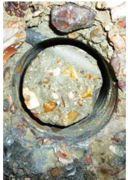
*Core sample extracted for laboratory testing.*
