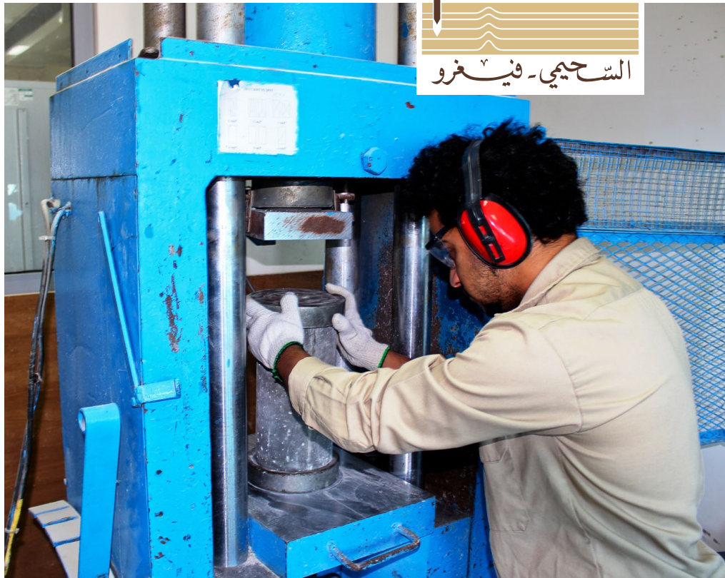
Determining the compressive strength of concrete cylinders.
