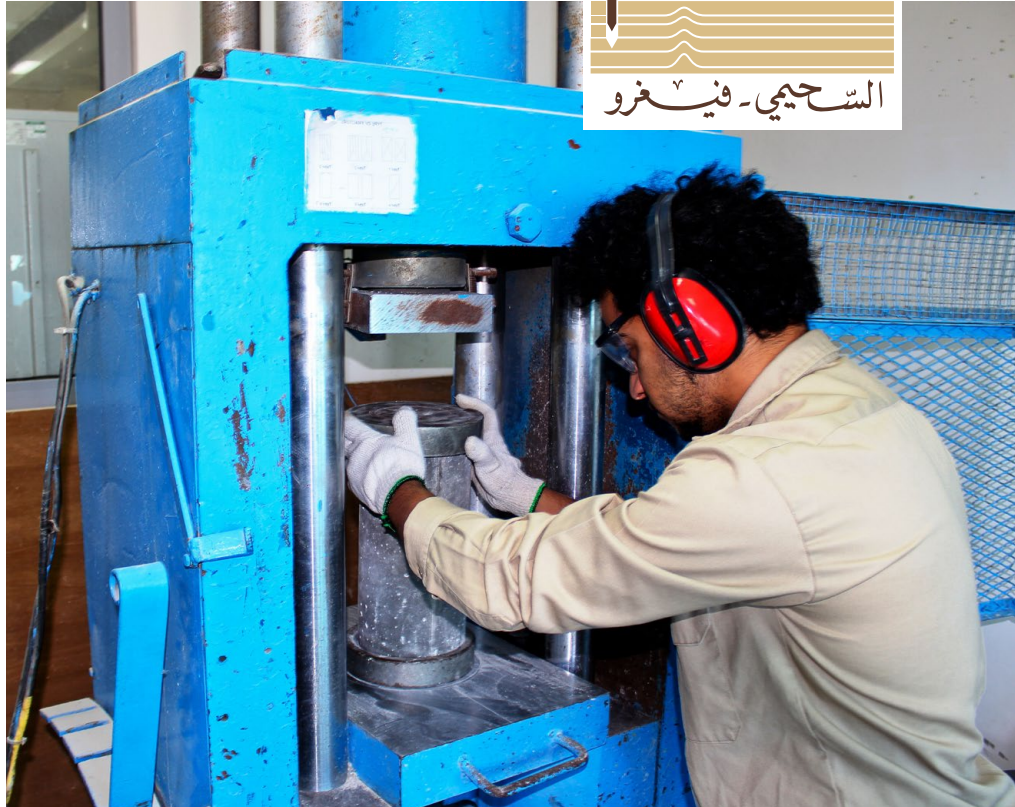
Determining the compressive strength of concrete cylinders.
