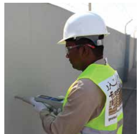
Rebound hammer testing of concrete.
