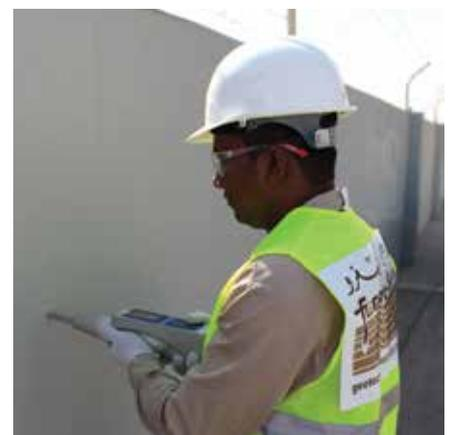
Rebound hammer testing of concrete.
