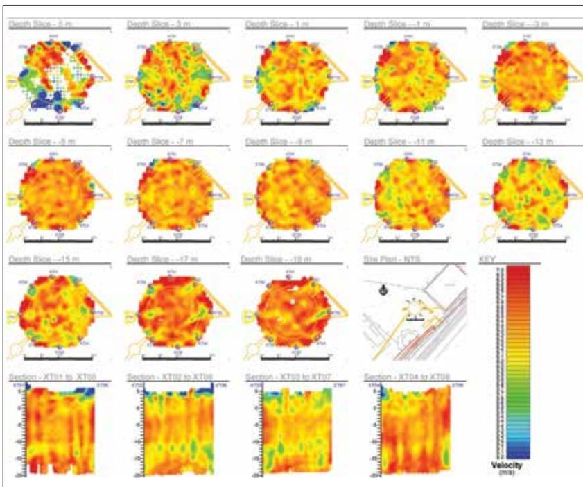
**Above:** Figure 2, 3D seismic tomographic imaging at multiple depths can be applied to planned shaft structures to verify the absence of potentially hazardous conditions such as faulting or voiding
