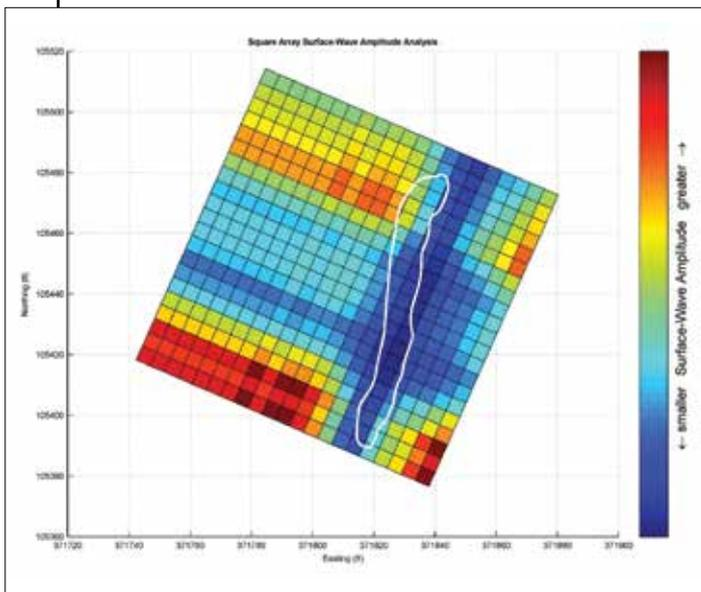
**Above: Figure 4, Square array void mapping (SAVM) uses an array of seismic sources to investigate a 3D volume of ground and is ideally suited to tunnel investigations in non-urban environments. Voiding (indicated by the white line) can be diagnosed from zones of anomalous amplitude and/or low seismic velocity**
