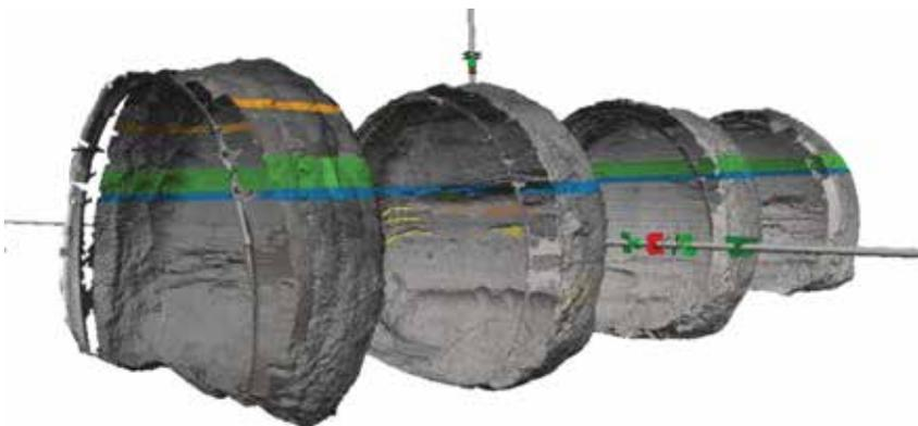
Above: Figure 5, Lidar imaging is an effective method for profile geometry and convergence analysis, excavation face mapping, and geological analysis combined with hyperspectral imaging
