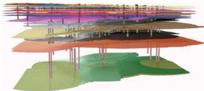
Above: Figure 1, The Final Integrated Ground Model provides a representation of geotechnical and hydrogeological properties, stratigraphy and geohazards
