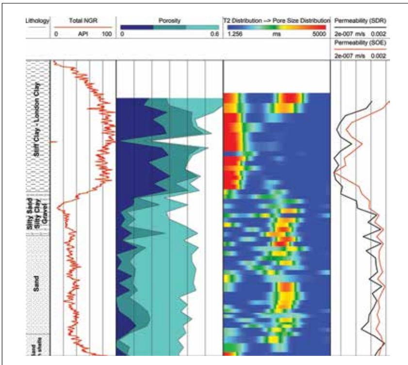
**Above:** Figure 3, The downhole magnetic resonance (DMR) method can yield in situ measurements of porosity and permeability in addition to quantifying bound and mobile water without pumping tests
