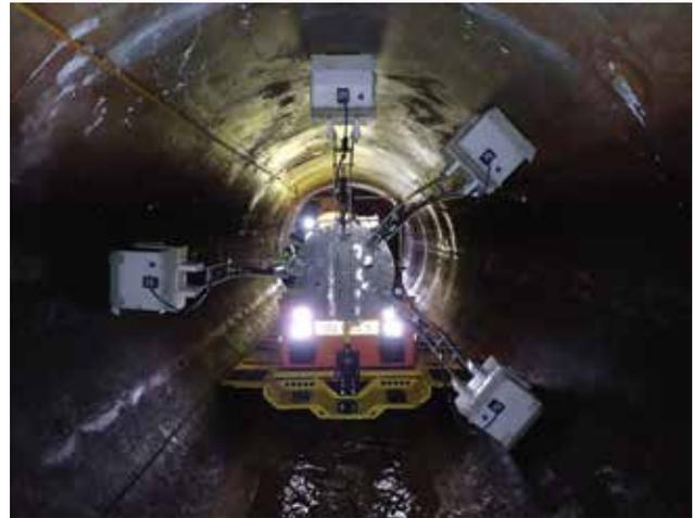
**Above:** Figure 6, Fugro developed a bespoke multi-channel ground penetrating radar system to survey 40 kilometres of concrete tunnels at Haweswater Aqueduct in NW England. More than 800 profile kilometres of data were collected in less than two weeks
