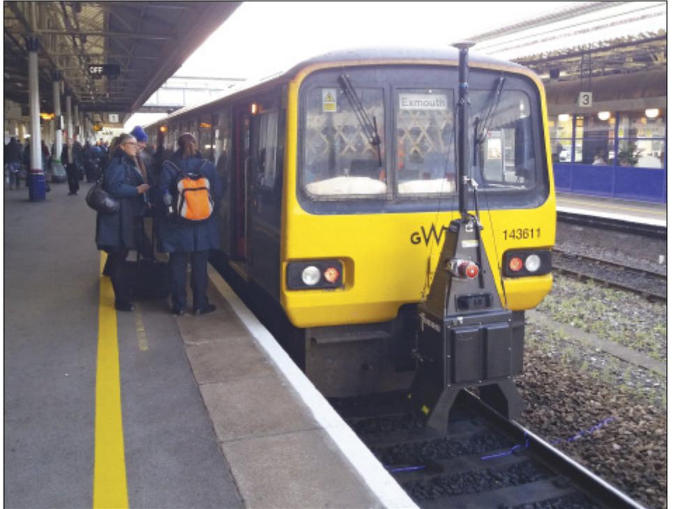
The RILA 3.0 system with integrated 360° scanner, high-resolution imaging and video cameras fitted to the rear of a timetabled passenger service. It projects a laser beam over the rail, as can be seen from the blue line on the track in front of the vehicle.
