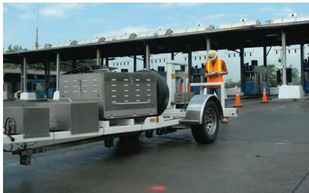
Pavement analysis using Falling Weight Deflectometer (FWD)
