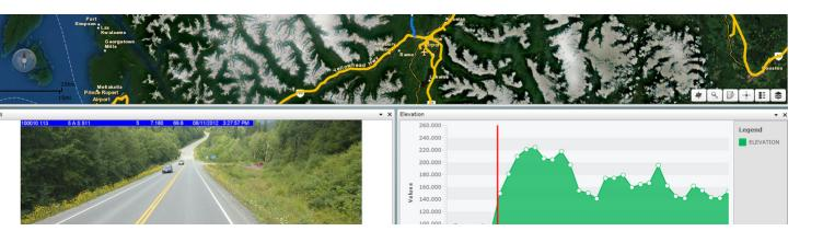
Fugro Smart Geometrics is a vehicle-mounted subsystem that utilizes a patented control algorithm and a combination of gyroscopes and software to measure the crossfall, transverse profile, vertical alignment (grade) and horizontal alignment (curve radius) of the roadway.
