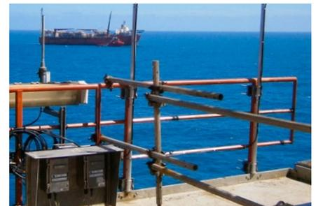
*Decommissioning application - platform motion monitoring equipment with satellite communication.*
