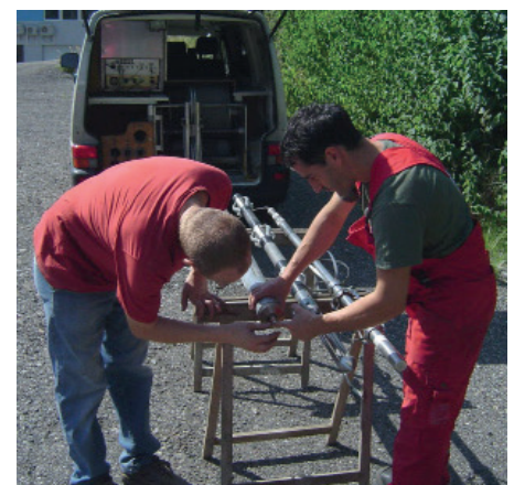
Off-site calibration of 4-arm-caliper tool
