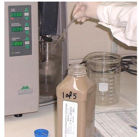
Preparing a sample for analysis using laser diffraction.
