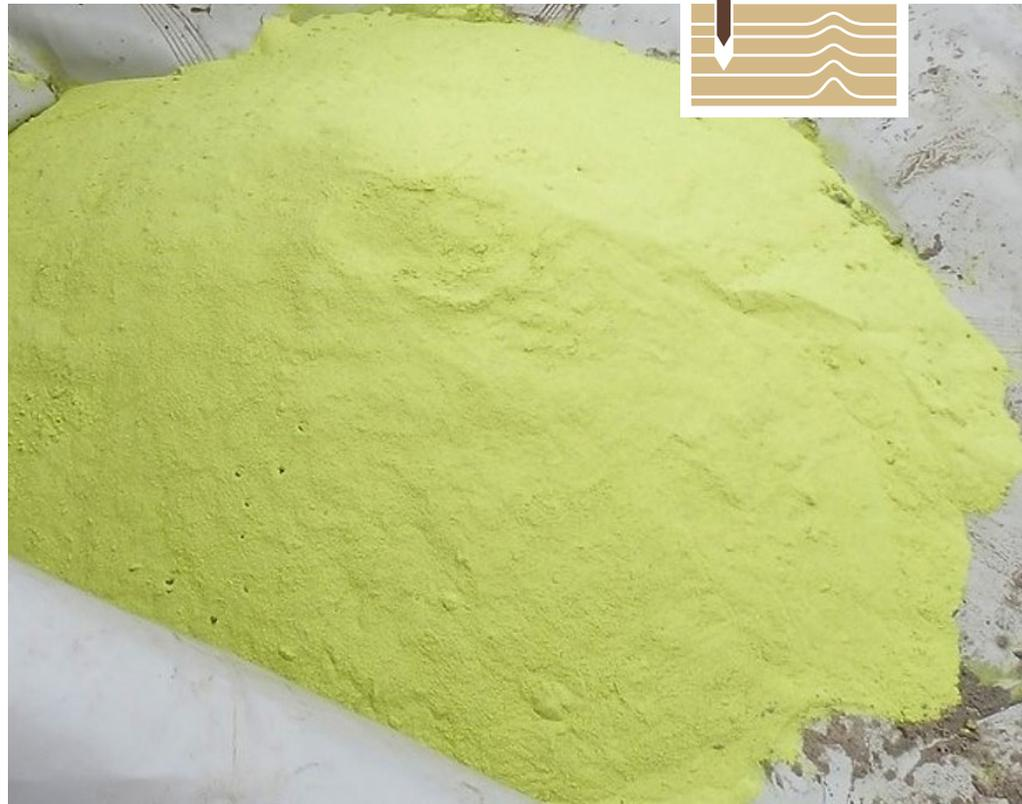
Concentrated tracer sediment prior to release into the environment.
