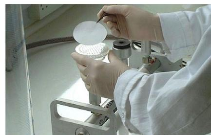
*Preparing equipment for total suspended sediment analysis.*
