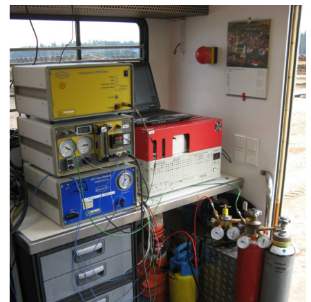
MIP controller and gas detector units
