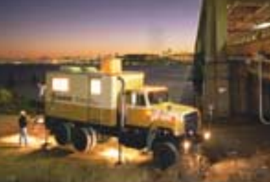
CPT truck in action near the San Francisco Oakland Bay Bridge.
