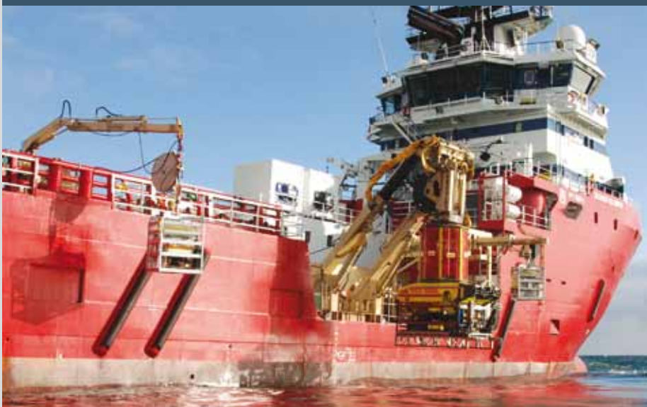
▼ the Skandi Olympia with 3 ROVs being deployed over the starboard side of the vessel
