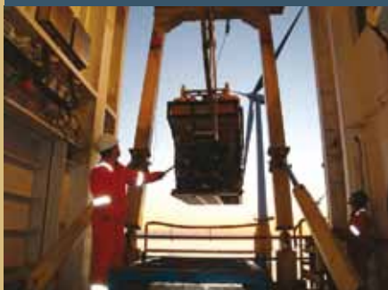
▼ Fugro Sealion ROV being launched from the Normand Mermaid
