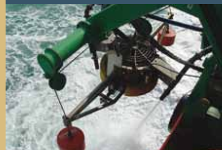
▼ Marin Subsea Vortex tool fitted with mono-jet to facilitate clay soil break up
