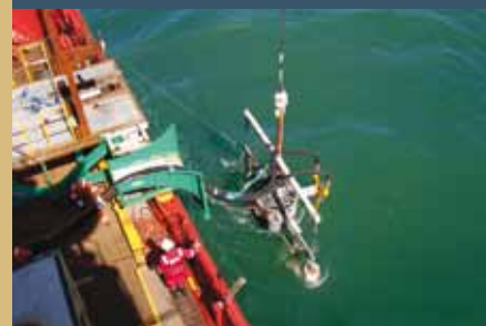
▼ Marin Subsea Vortex tool fitted with mono-jet to facilitate clay soil break up
