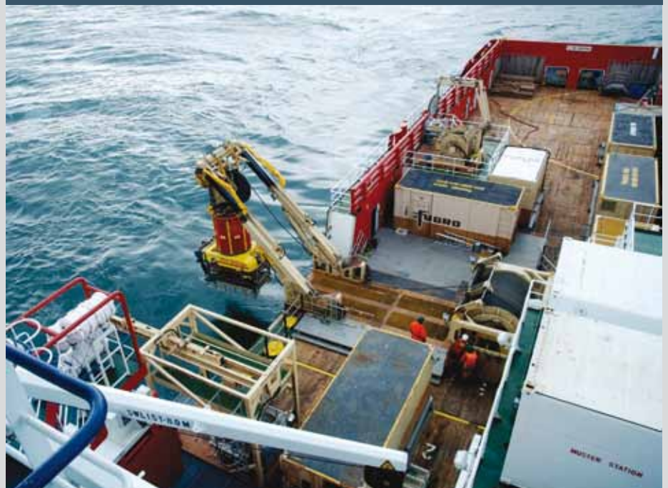
▼ view showing, the Crane deployed Tiger inspection ROV at the aft end, the 'A' Frame deployed FCV 3000 Work-class ROV centre and the beam deployed Tiger nearest
