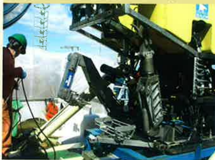
▼ Sealion 14 fitted with specialised repair tools
